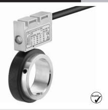
Thanks to its installation depth of only 16 mm, the bearingless magnetic rotary encoder RI20 / Limes LI20, comprising a magnetic ring and sensor head, is ideally suited for plants and machinery where space is very tight. The non-contact measuring principle allows for error-free use even under harsh environmental conditions, as well as ensuring a long service life.
