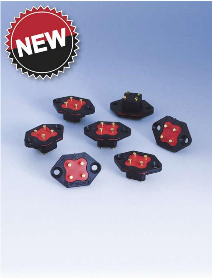
Our new NF04 BL0-Series connector has a rugged design particularly suitable for use in battery-powered equipment. Connector NF04 BL0 is meant for mounting within the piece of equipment, e.g. in its battery case. When inserting the battery pack the connector gets engaged by means of the battery terminals. Equipped with spring contacts the connector features a steady low contact resistance.
