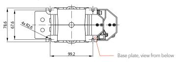
The contactors are mounted on a suitable mounting plate with four M5 screws.
