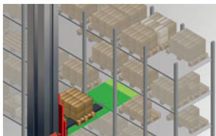
Space check and collision prevention during storage by shelving storage and retrieval units
