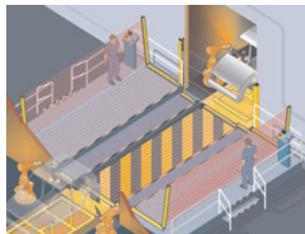
Point-of-operation guarding with M4000 Area at an output conveyor in the automotive industry
