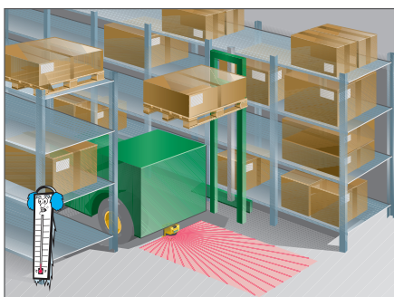
Hazardous area protection in cold storage with S3000 Cold Store
