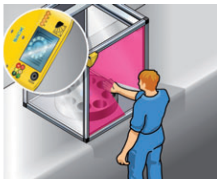
Hazardous point protection on a semi-automatic assembly machine
