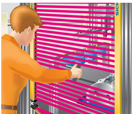
Printing industry: C2000 Cascadable on a pad printing machine
