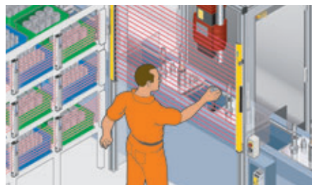
Parts supplier industry: Hazardous point protection at assembly machine
