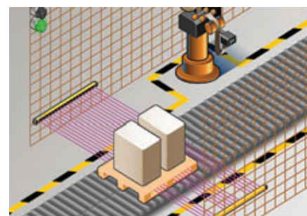
Sensor differentiates between pallets and worker
