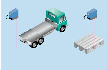
$\ \, \blacktriangle$  A variant of the sensor, used to detect objects between the sensor and a fixed background.
