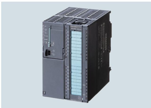
The SIWAREX FTC (Flexible Technology for Continuous Weighing) is a versatile and flexible weighing module for conveyor scales, loss-in-weigh scales and bulk flow meters. It can also be used to record weights and measure force. The SIWAREX FTC function module is integrated in SIMATIC S7/PCS7, and uses the features of this modern automation system, such as integral communication, diagnostics and configuration tools.
