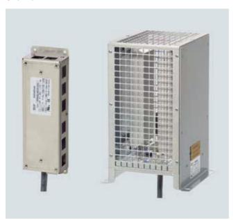
Excess power in the DC link is dissipated via the braking resistor. The braking resistors are intended for use with PM240 Power Modules which feature an integrated brake chopper, but cannot regenerate energy to the supply system. For regenerative operation, e.g. the braking of a rotating mass with high moment of inertia, a braking resistor must be connected to convert the resulting energy into heat.
