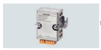
The Safe Brake Relay allows the Power Module to be safely connected to an electromechanical motor brake, allowing the brake to be directly and safely controlled by the Control Unit in accordance with EN 954-1, safety category 3, and IEC 61508 SIL 2.
