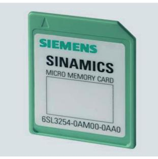
The parameter settings for an inverter can be stored on the MMC memory card. When the plant is serviced, it is immediately ready for use again after, for example, replacement of the frequency inverter and transfer of the memory card data. The associated slot is located on the rear of the Control Unit.
