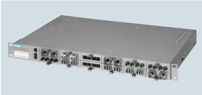
The SCALANCE XR-300 Industrial Ethernet switches are fully modular, high-performance, industry-standard switches for the construction of electrical and optical line, ring and star topologies with data transfer rates of 10/100/1 000 Mbit/s, designed for installation in 19" control cabinets.
