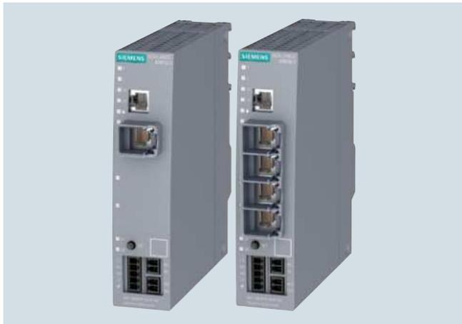
The SCALANCE M812-1 and M816-1 are DSL routers for low-cost and secure connection of Ethernet-based subnets and programmable controllers to wired telephone or DSL networks and support ADSL2+ (Asynchronous Digital Subscriber Line). This allows the devices to have high downlink data rates of up to 25 Mbit/s and uplink data rates of up to 3.5 Mbit/s.
