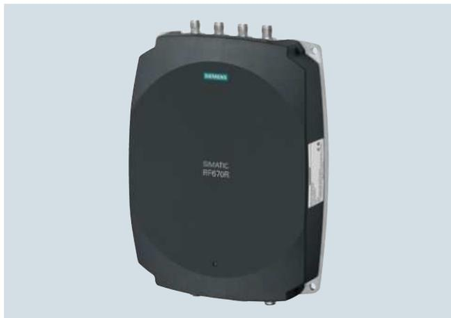
SIMATIC RF670R is a high-performance RFID reader with four antenna connections which can be configured as required for individual read stations, detecting at conveyor systems, or as gates. The high transmit power of up to 2 W ERP / 4 W EIRP (dependent on antenna and cable) permits large ranges of up to 10 m in gate applications. The high degree of protection of the overall system is a guarantee for problem-free use, even under the most difficult environmental conditions.
