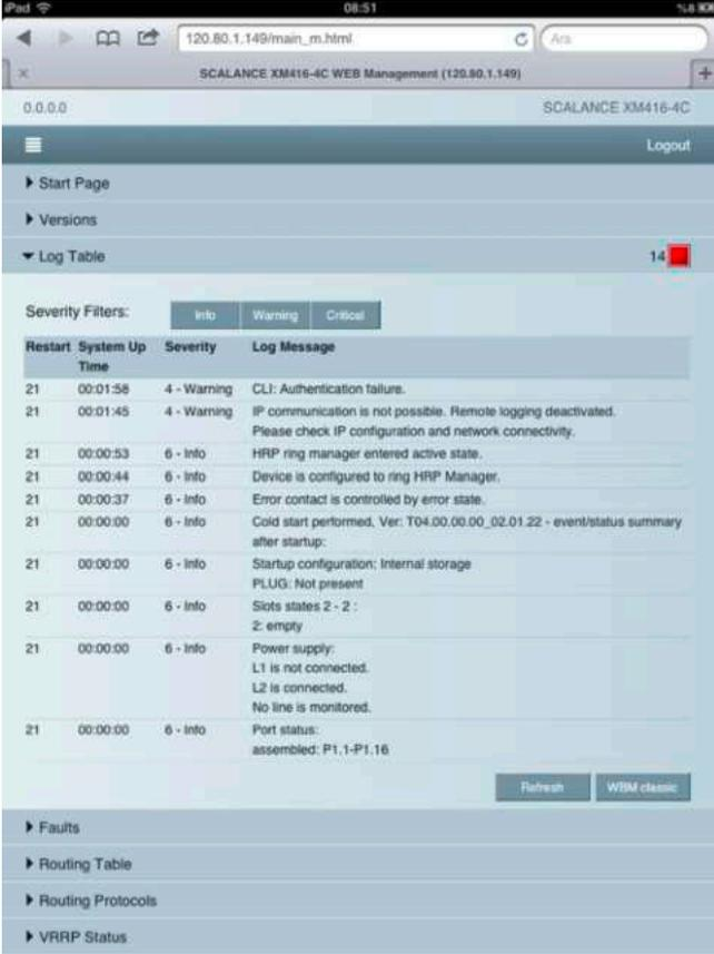
The screenshot shows the web management interface for a SCALANCE XM416-4C switch. The page title is "SCALANCE XM416-4C WEB Management (120.80.1.149)". The main content area displays a "Log Table" with 14 entries. The table has columns for "Restart Time", "System Up Time", "Severity", and "Log Message". The severity filters are set to "Info", "Warning", and "Critical".
