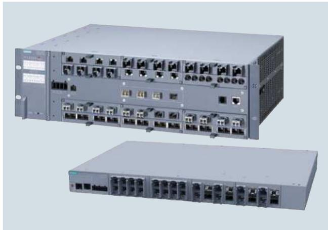
The Layer 3-enabled SCALANCE XR-500 Industrial Ethernet switches are fully modular, high-performance, industry-standard switches for the construction of electrical and optical line, ring and star topologies with data transfer rates of up to 10 Gbit/s, designed for installation in 19" control cabinets.
