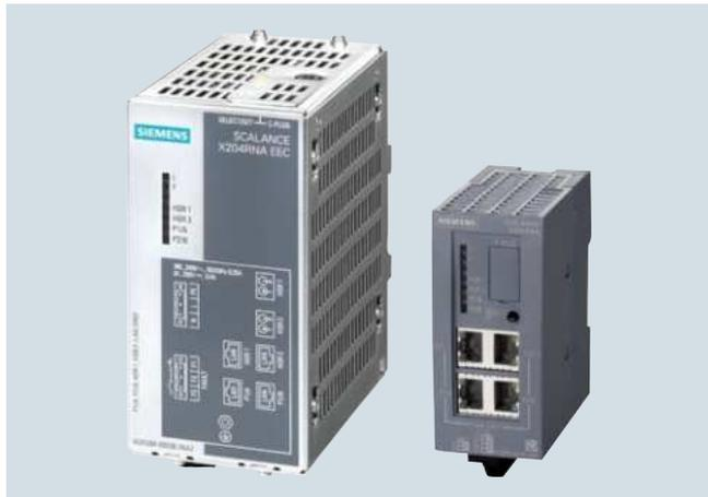
The SCALANCE X-200RNA (**R**edundant **N**etwork **A**ccess) managed Industrial Ethernet network access points with HSR functionality (**H**igh-availability **S**eamless **R**edundancy Protocol in accordance with IEC 62439-3) are used to connect up to two non-HSR-enabled terminal devices or network segments to a ring-shaped HSR network structure. They can also be used for simple and redundant transition from HSR to PRP (Parallel Redundancy Protocol) network structures.
