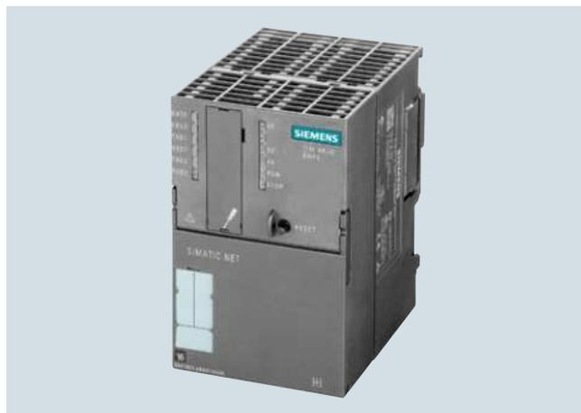
The TIM 4R-IE DNP3 (DNP3 protocol) has two RS 232/RS 485 interfaces for data transmission via conventional WANs (copper dedicated line, analog dialup modems, wireless) and two additional RJ45 interfaces for connection to IP-based networks (WAN or LAN).
