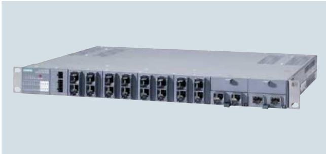
The SCALANCE XR-300PoE Industrial Ethernet switches are partly modular, high-performance, industry-standard switches for the construction of electrical and/or optical line, ring and star topologies at data transfer rates of 10/100/1 000 Mbit/s, designed for installation in 19" control cabinets
