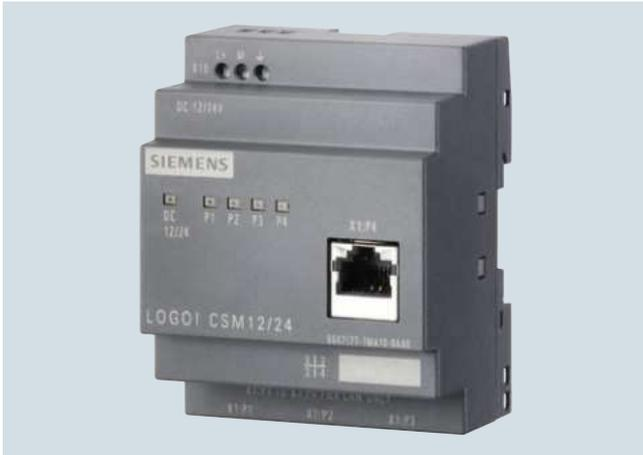
The module is used to connect a LOGO! and up to three other nodes to an Industrial Ethernet network with 10/100 Mbit/s in an electrical linear, tree or star topology.
