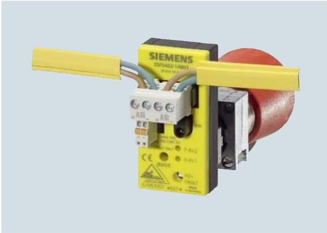
The AS-Interface F adapter is used to connect an EMERGENCY-STOP device according to ISO 13850 from the 3SB3 series to the AS-Interface bus system. The F adapter is suitable for control devices with mounting on front plates.
