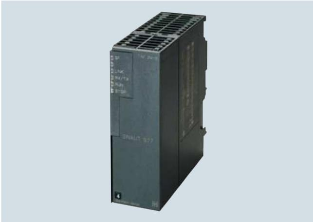
The TIM 3V-IE is a SINAUT communications module for the SIMATIC S7-300. It has an RS232 interface to which a matching external modem can be connected for data transfer via a conventional WAN. It additionally possesses an RJ45 interface, which permits communication over IP-based networks. In the case of the TIM 3V-IE, SINAUT communication can be processed alternately via one of the two interfaces, while in the TIM 3V-IE Advanced both interfaces can be operated simultaneously.
