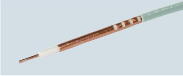
The RCoax cables are radiating cables that function as special antennas for the SCALANCE W Access Points in environments with complex radio coverage. Its design means that a defined, cone-shaped radio field is generated along the RCoax cable. The radiating cables are therefore perfectly suitable for use in all types of applications with track-bound vehicles.
