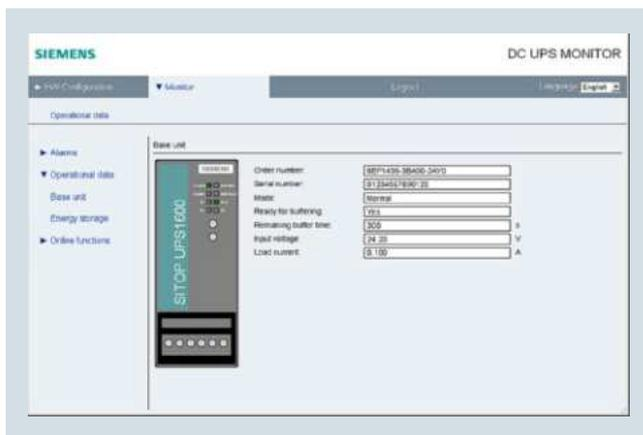
The password-protected web server supports viewing of the configuring and operating data.
