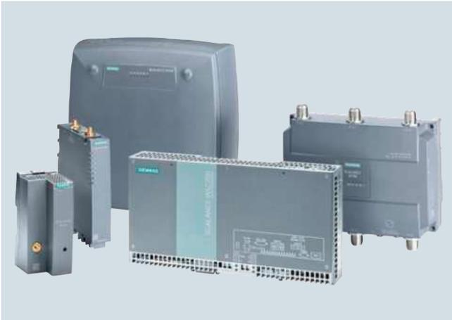
The access points of the SCALANCE W700 product lines are ideally suited for setting up Industrial Wireless LANs (IWLAN) for 2.4 GHz or 5 GHz. They can be used in all applications that require a high degree of operational reliability, even in extremely harsh surroundings.
