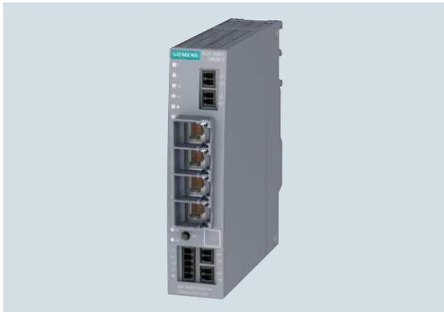
The SCALANCE M826-2 is an SHDSL modem for low-cost, secure connection of Ethernet-based subnets and programmable controllers via existing two-wire or stranded cables and supports the ITU-T standard G.991.2 as well as SHDSL.biz (single-pair high-speed digital subscriber line). This gives the device high symmetrical data rates of up to 15.3 Mbit/s per wire pair.
