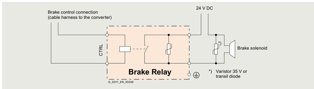
Connection example of 24 V DC Brake Relay
