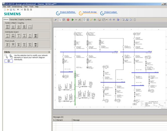
SIMARIS design is a planning tool for quick and effective network calculation and dimensioning of power distribution for non-residential and industrial buildings.
