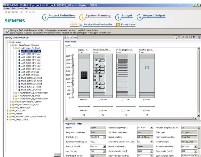
SIMARIS project is a planning tool for fast calculation of space requirements and electrical power distribution system budgets for non-residential and industrial buildings, and for generating specifications automatically.
