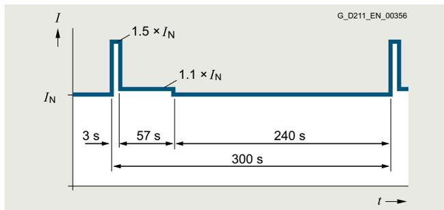
300 s duty cycle based on low overload
