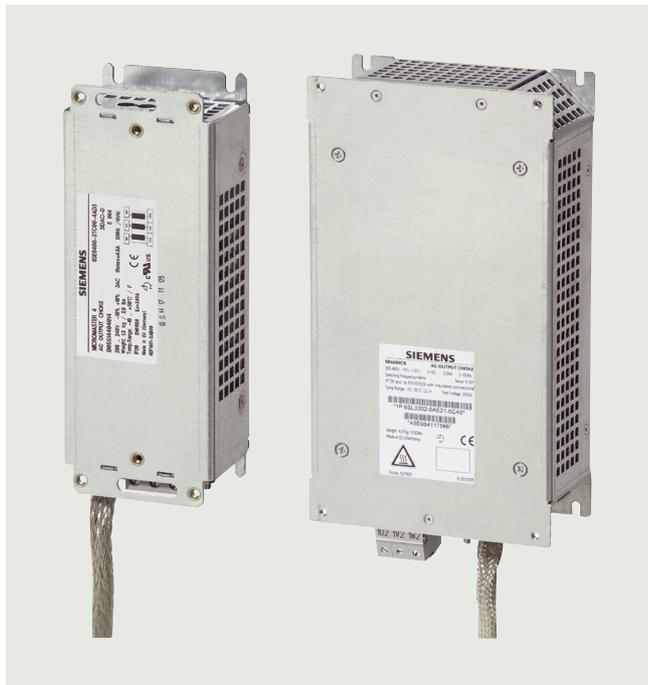
Output reactors reduce the voltage stress on the motor windings. At the same time, the capacitive charging/discharging currents, which place an additional load on the power unit when long motor cables are used, are reduced.
