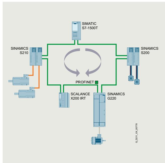
Bumpless media redundancy illustrated by example of SINAMICS G220, S200, S210 and SCALANCE X200IRT
