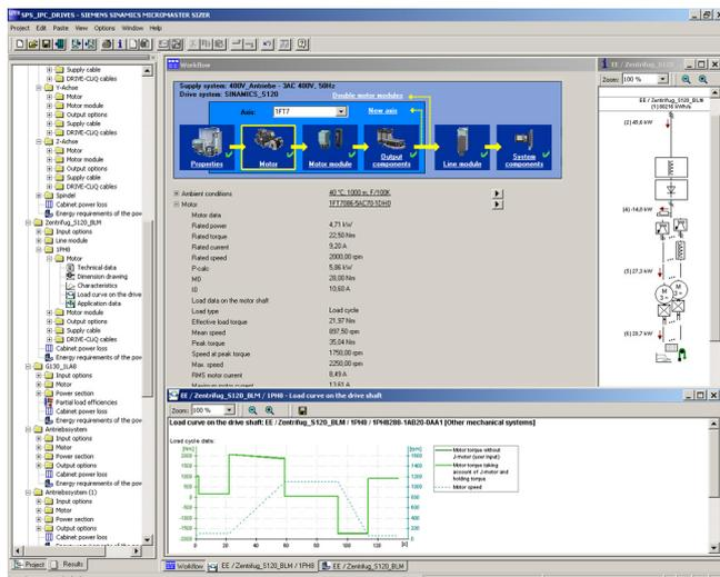
The following drives and controls can be engineered in a user-friendly way using the SIZER for Siemens Drives engineering tool:
