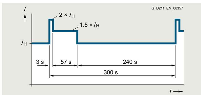
300 s duty cycle based on high overload
