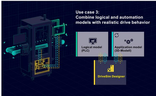
With the third Use case, you can connect a simulation tool such as NX Mechatronic Concept Designer to visualize the mechanical movements of your application. This way, you ensure that the drive behaves according to the desired machine performance. You can test several fault scenarios and optimize the interaction between PLC, application and drive virtually so overall, you can avoid unplanned machine behavior and increase the performance of your setup.
