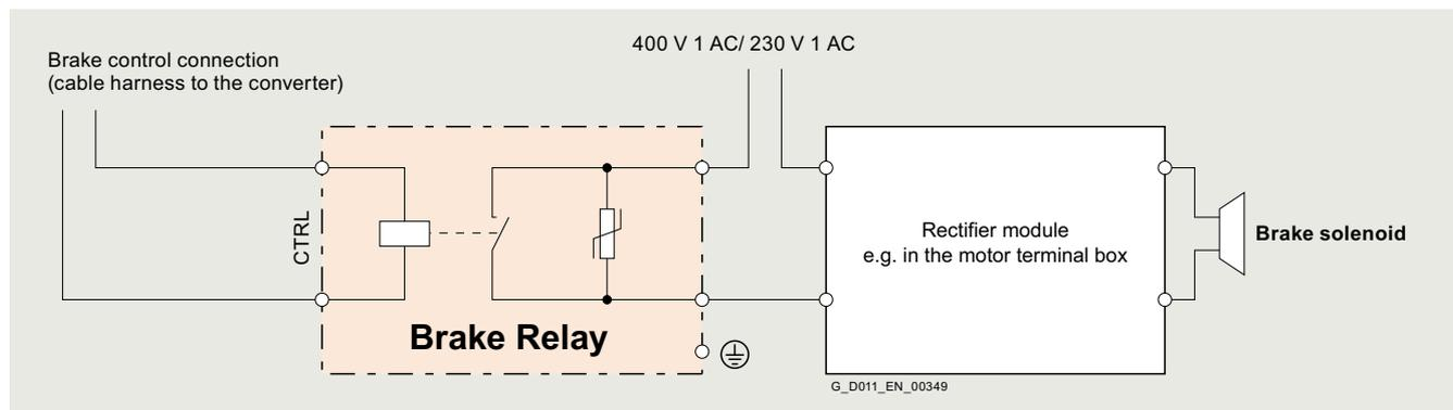
Connection example of 230 ... 400 V 1 AC Brake Relay
