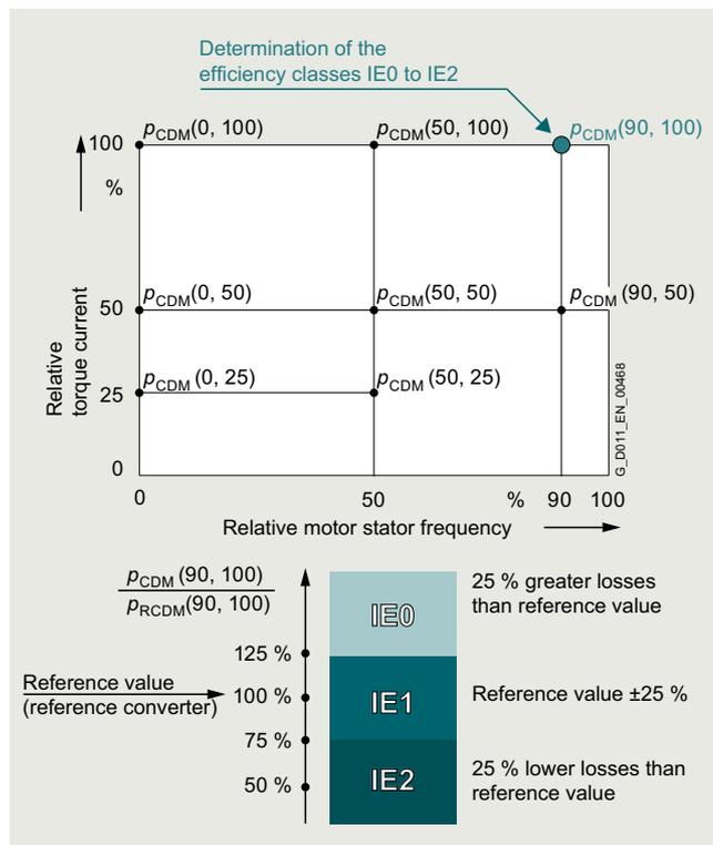
Complete Drive Module (CDM) – determining the efficiency class
