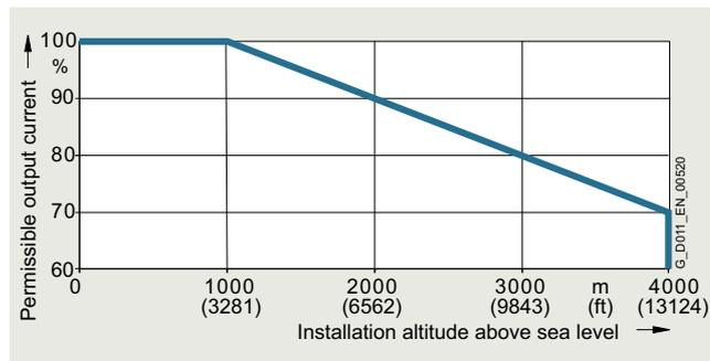
Permissible output current as a function of the installation altitude for PM240-2 Power Modules at 40 °C for low overload (LO)
