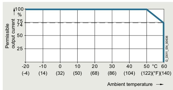
Permissible output current as a function of ambient temperature for high overload (HO) for PM240-2 Power Modules
