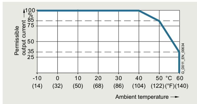
Permissible output current as a function of ambient temperature for low overload (LO) for PM240-2 Power Modules
