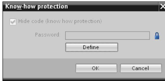
Figure 11-5 Setting up block know-how protection (2)
