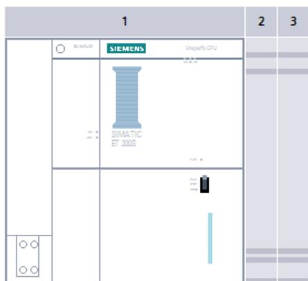
Figure 9-1 Unspecified CPU in the device view
