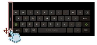
To move the floating screen keyboard, drag the floating keyboard by its left bar to the desired position.
