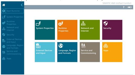
2. If desired, operate the project or configure the HMI device via the Control Panel. If you no longer need the HMI device, switch it off.
