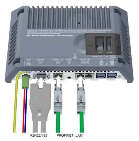
Use the PROFINET (LAN) X1 or X2 interface for SIMATIC process connection. Only use the RS 422/485 interface for controllers from other manufacturers that are connected in conjunction with a CSP on the serial interface. Additional information on compatible controllers is available in the section "Communication with controllers (Page 184)".
