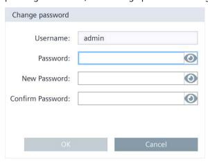
Enter the previous password once and the new password twice. The following button can be used to make the passwords visible for the display duration of the dialog box:
