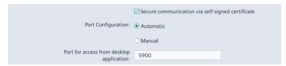
• "Secure communication via self-signed certificate": Option to enable secure communications via SSL encryption. Default setting: "activated".
