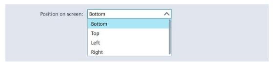
"Position on screen": Drop-down list to specify the position of the taskbar on the display. The drop-down list is only active when the "Enable taskbar" option is selected.
