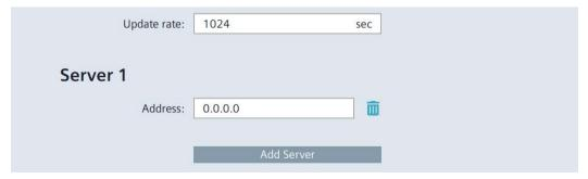
Enter the desired synchronization interval under "Update rate", value range 10 to 86400 seconds (1 day). After the input, the value is rounded to the nearest power of two based on the internal format.
