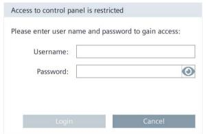
Log in as a user with the "Control Panel access" function right to activate the password protection for the Control Panel. Use the following button to make the password visible for the display duration of the dialog:
