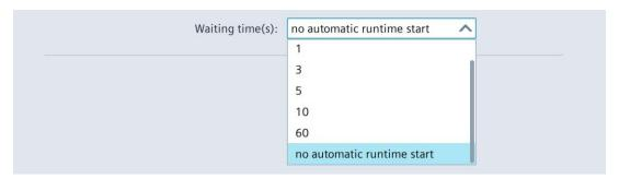
"Waiting time(s)": Drop-down list for determining whether the project on the HMI device starts automatically after a specified delay time or not.
