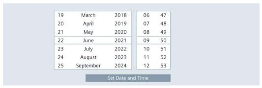
Set the day, month, year and time by scrolling the respective list column so that the desired date and time are displayed in the framed line in the middle of the list. The "Set Date and Time" button is used to save the setting.
