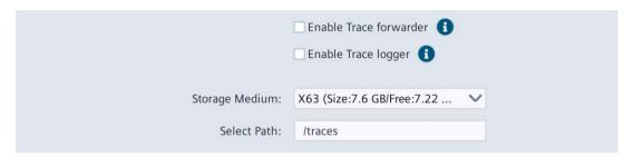
• "Enable Trace forwarder": Option to enable or disable the "tracing" service. The default setting is "deactivated".
