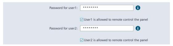
In this area you define the passwords and access rights for two users. The passwords of the two users must not be identical. Several users can access the SmartServer simultaneously via one password.
