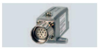
SME20/SME25 Sensor Modules External are encoder evaluation units for machine encoders (direct measuring systems). The devices are designed with IP67 degree of protection. This means that the units can be installed outside the control cabinet near the machine encoder.
