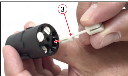
Assembly of whole filler plugs (3) for socket inserts
