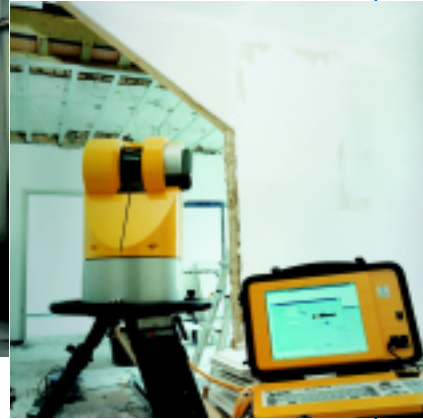
Use in building as a contour measurement system
