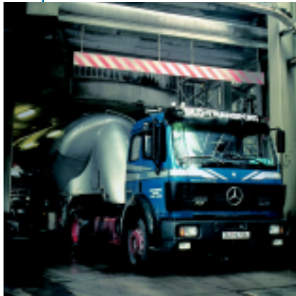
Positioning aid for silo vehicles for precise loading
