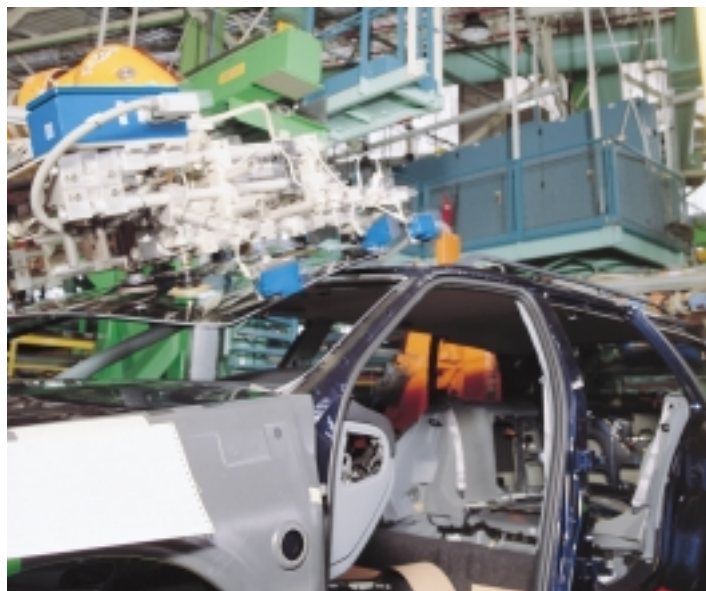
▼ In a car factory, WT 30 sensors being used to ensure that windscreens are precisely positioned before they are bonded to the vehicle body.
