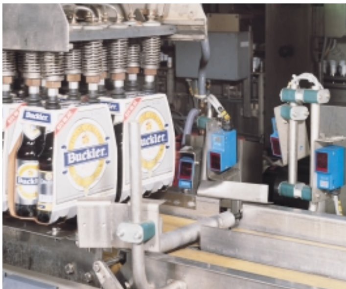
▲ WT 30 used to check the presence of six-packs.
