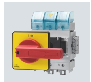
3LD2 217-1TL13 switch for floor mounting, 250 A, with rotary operating mechanism and door coupling
