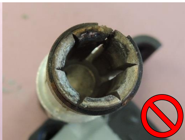
Socket contact contaminated due to the effect of acid
