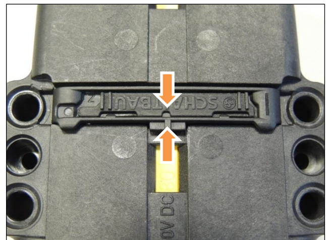
Image 6: Slider with a lock in the locked condition, Recess and the crossbar are located above each other (see the arrows)
