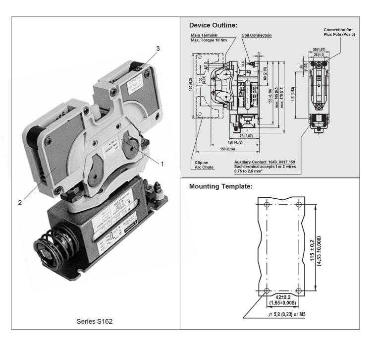
Contact (Pos.1) and arc chute (Pos. 2) can be easily replaced if necessary (for part No. see page 9). Keying prevents reverse insertion of the arc chute.
